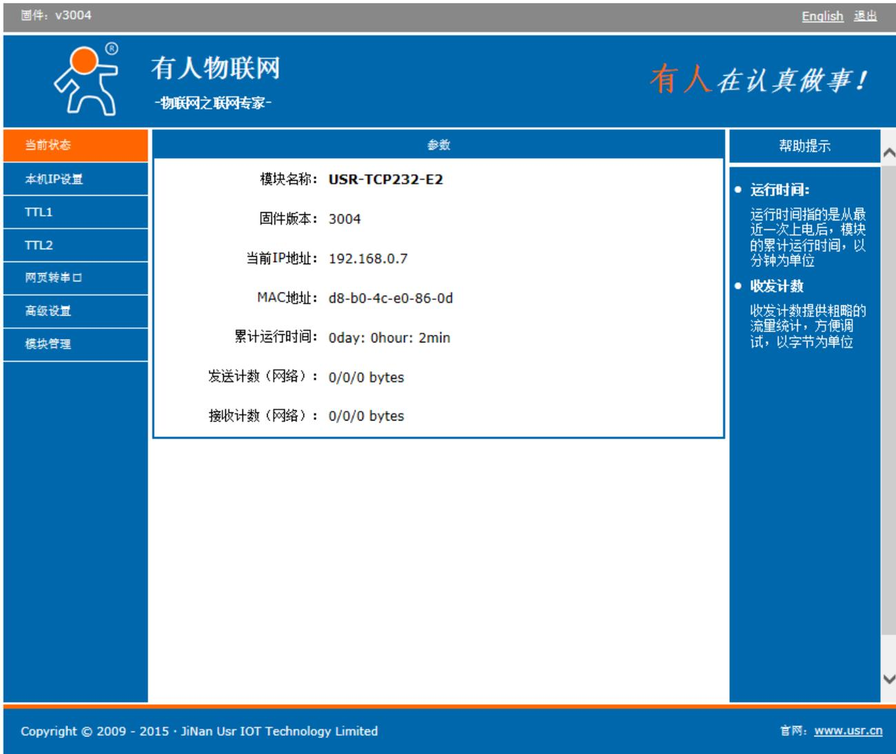
The screenshot displays the web management interface for the Usr-TCP232-E2 module. The interface is in Chinese and includes a sidebar with navigation options like '本机IP设置', 'TTL1', 'TTL2', '网页转串口', '高级设置', and '模块管理'. The main content area shows the following parameters:
